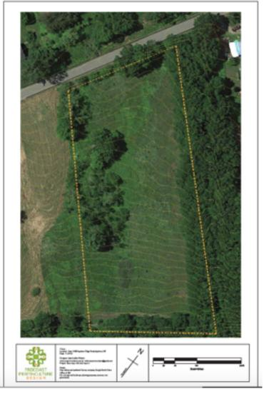
Some base maps include multiple layers like color aerial photos, property boundaries and topographical data. Design work then proceeds as overlay images. This example is 24x36 or Arch D sized paper.
